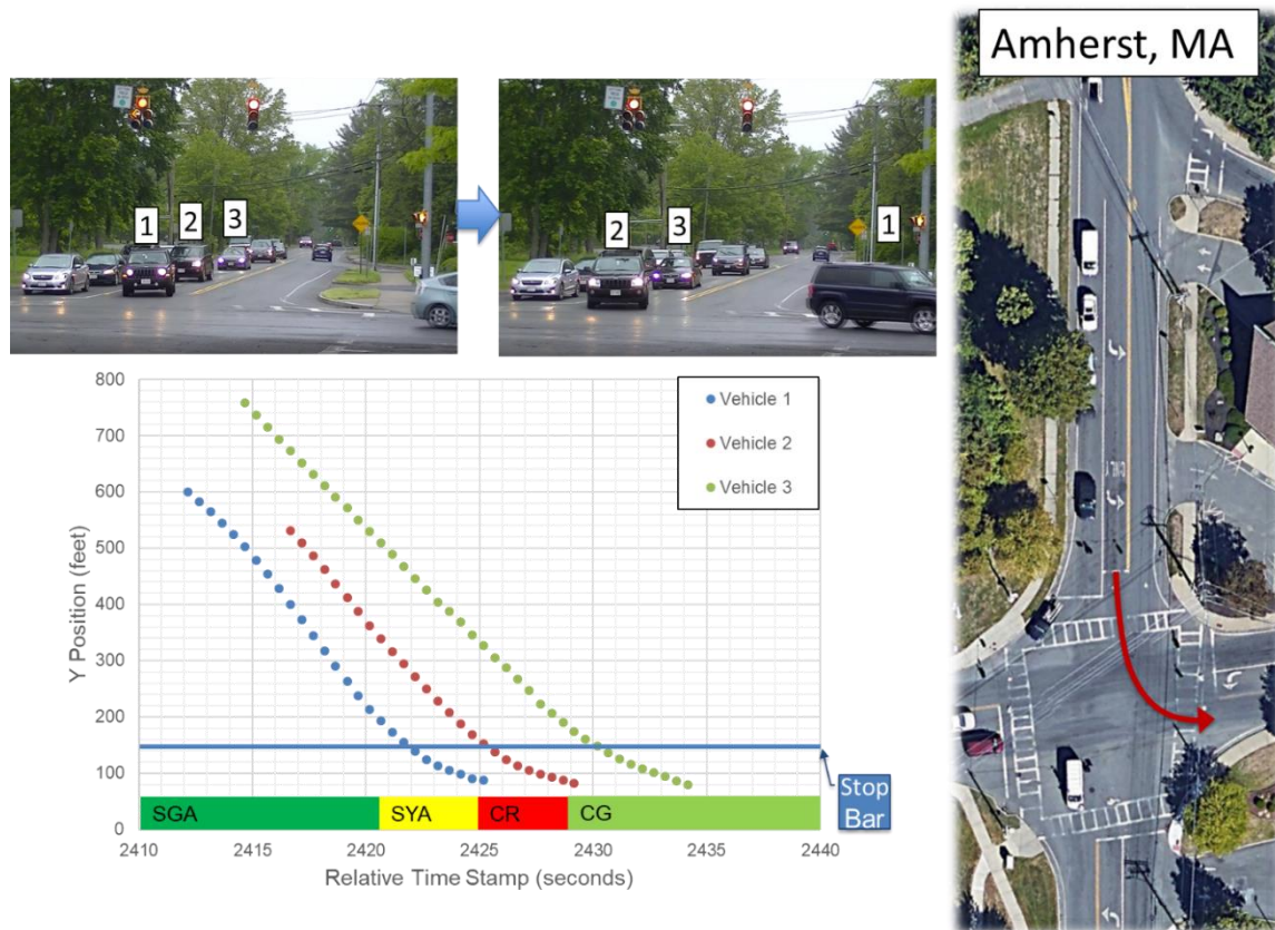
Figure 4.17 – Vehicles using all-red as extension of protected phase in CG PPLT.
