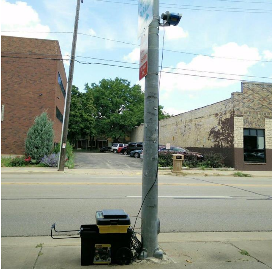
Figure 3.3 – Mobile deployment of trajectory data collection system.
